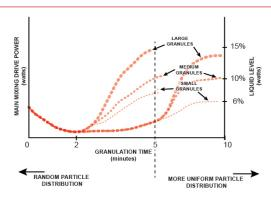
In Processall's Mixmill® line of mixing granulators, mediumdensity blending elements lift and disperse the product to produce a mechanically fluidized bed, which rapidly and efficiently blends materials of widely different density and particle size, while an integral high-intensity chopping mill system distributes the agglomerating solutions while binding and controlling particle size. Post milling is usually unnecessary.
