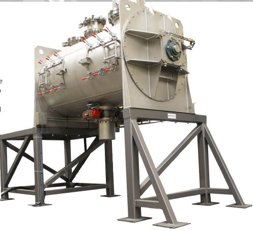
with adjustableweirs are provided to introduce the product through different processing zones for thermal treatment or conducting chemical reactions. The device incorporates a heating or cooling jacket.
