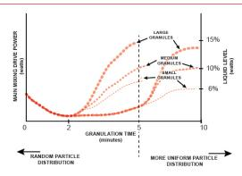
In Processall's Mixmill® line of mixing granulators, mediumdensity blending elements lift and disperse the product to produce a mechanically fluidized bed. This rapidly and efficiently blends materials of widely different density and particle size. Meanwhile an integral, high-intensity chopping mill system distributes the agglomerating solutions while binding and controlling particle size. Post milling is usually unnecessary.
